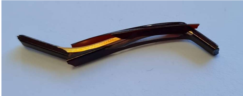
Figure 8-6. Evidence of conductor/insulation separation during tests at 220°C for one week.
