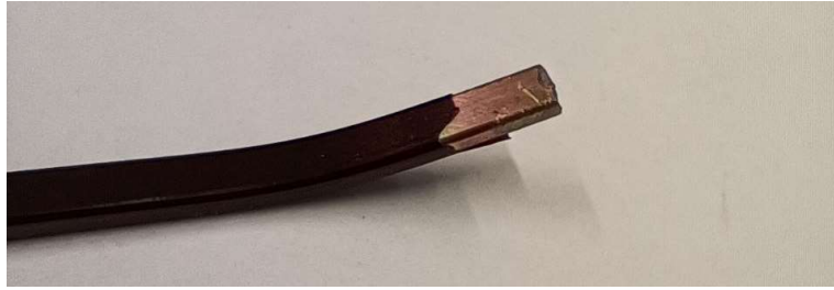
Figure 8-5. Evidence of conductor/insulation separation during the chemical compatibility tests
